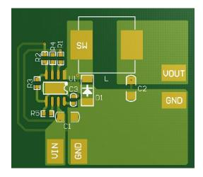
Figure 1. PCB Layout Recommendation
